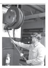
**HOSE OR CABLE BALL STOPS.** Except for 'constant tension' applications where the end of the hose or cable is tethered or otherwise secured, it is recommended that a ball stop, properly sized so the stop is larger than the roller assembly opening, be used in conjunction with your Hannay reel.
